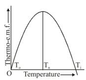
increases with the temperature of hot junction and becomes maximum at a particular temperature. The temiperature of the hot junction at which thermo e.m.f., in a thermocouple is maximum is known as neutral temperature  $T_n$  for that couple.
