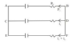
From FFBAE,  $i_1 R_1 + (i_1 + i_2) R_3 = E_1$
