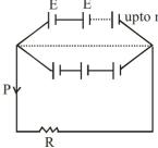
The current i in the circuit will be maximum when the factor ( m R+ n r) in the denominator is minimum. The denominator is minimum when mR = n r
